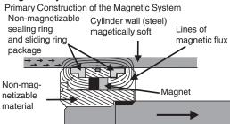
For this sensor principle it is not sufficient to simply mount the permanent magnet onto the piston. A magnetic system has to be constructed which conducts the magnetic flux of the permanent magnets directl into the cylinder wall in order to achieve the strongest possible magnetization. For further details regarding the construction of magnetic systems, refer to the manual. A field trial is generally recommended before practical operation!
